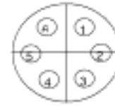
RS-232-cable (View of the CAMAT housing)
